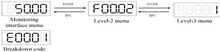
Figure 4-4 Operation hierarchy diagram of level of verify menu
