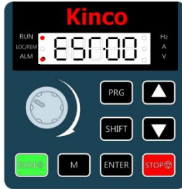
Figure 5-29 Self learning mode operation panel
