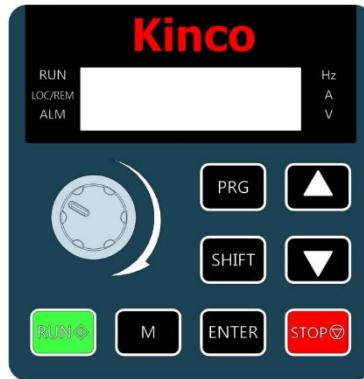
Figure 4-1 Schematic diagram of the LED operating panel
