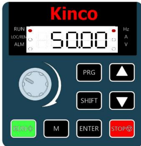
Figure 4-7 Steady operation display of the AC drive
