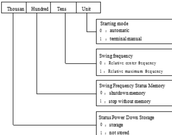
Fig. 6-57 Swing Frequency Operation
