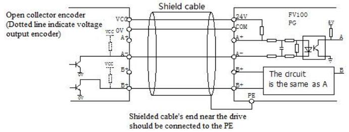
Fig.4-18 Wiring of open collector output encoder
