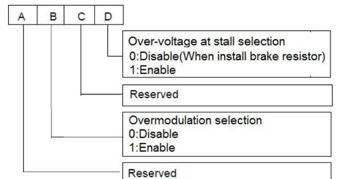
During deceleration, the motor's decelerate rate may be lower than that of drive's output frequency due to the load inertia. At this time, the motor will
