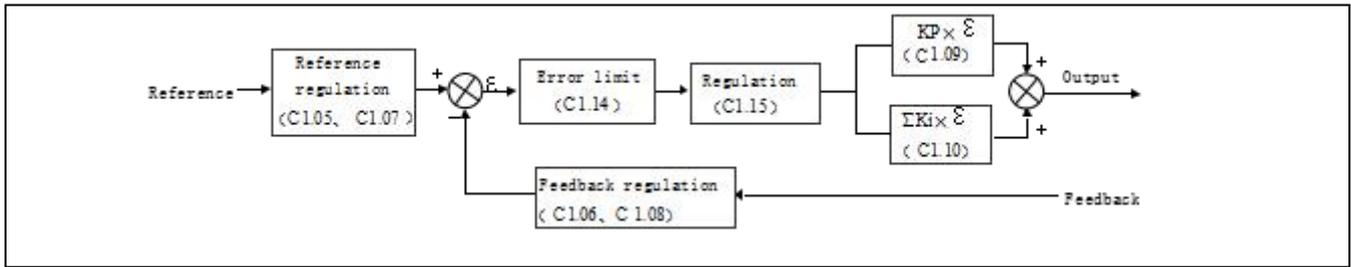
Fig.6-41 Principle diagram of process close-loop control
