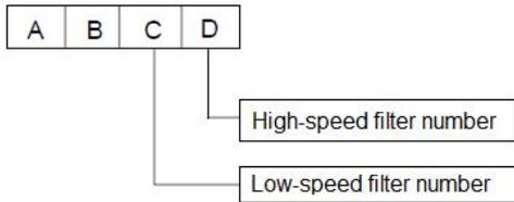
Increase the low-speed filter number if there is current noise when running at low speed, or decrease the low-speed filter number to enhance the system's response.
