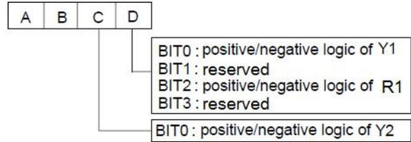
Fig.6-25 Output terminal's positive and negative logic
