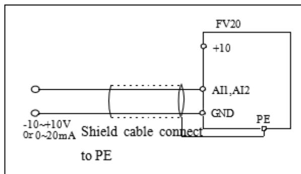
Fig 4-3 AI1 , AI2 terminal wiring
