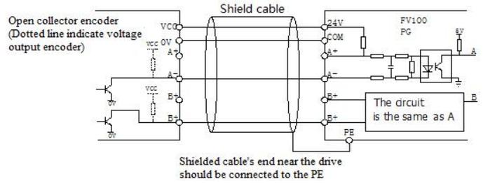
Fig.4-18 Wiring of open collector output encoder
