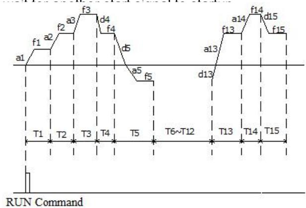
Fig.6-47 Stop after single cycle
