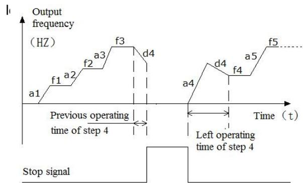
Fig.6-51 Start mode 2 of PLC function
