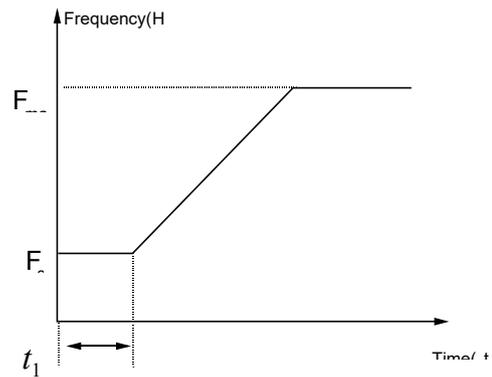
Fig.6-3 Starting frequency and starting time
