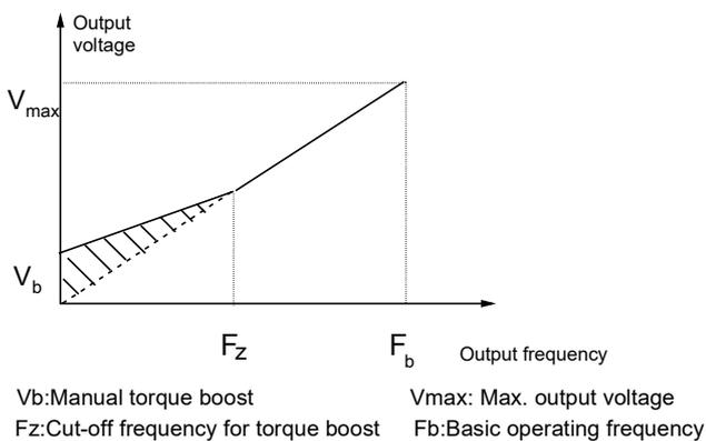
Fig.6-2 Torque boost
