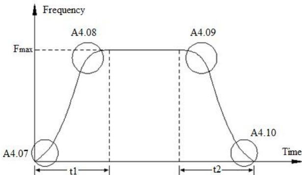
Fig.6-14 Acc/Dec starting time and ending time
