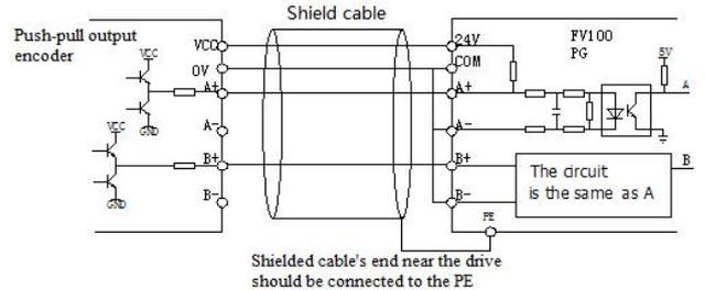
Fig.4-19 Wiring of push-pull output encoder
