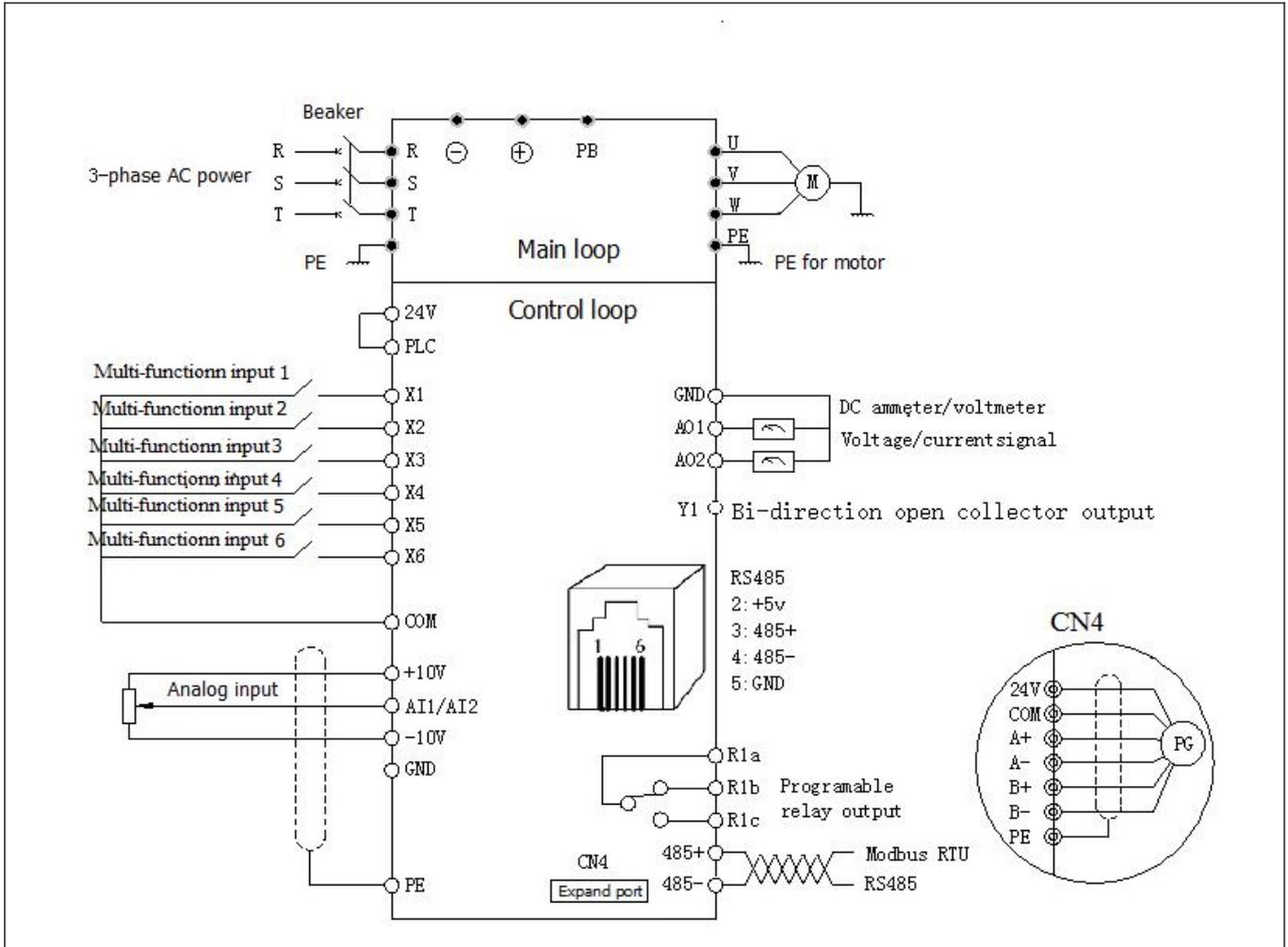
Fig.4-1 Basic wiring chart
