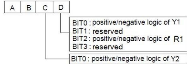
Fig.6-25 Output terminal’s positive and negative logic
