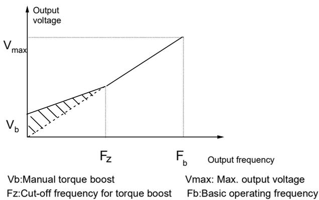
Fig.6-2 Torque boost
