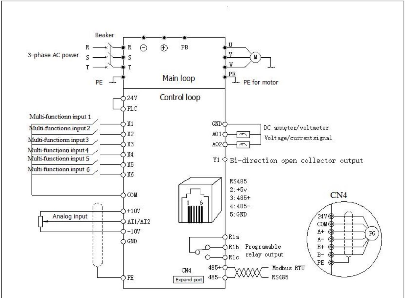
Fig.4-1 Basic wiring chart
