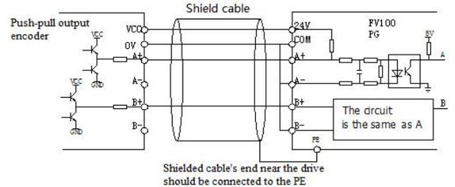
Fig.4-19 Wiring of push-pull output encoder
