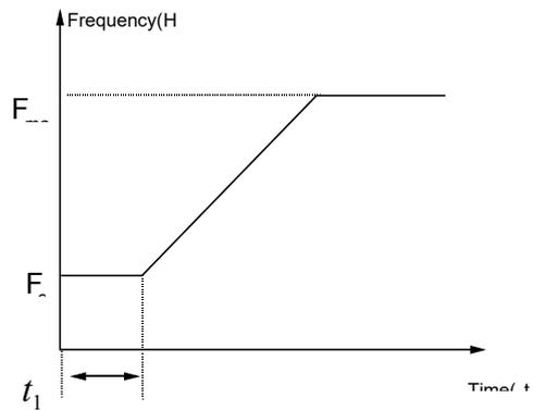
Fig.6-3 Starting frequency and starting time
