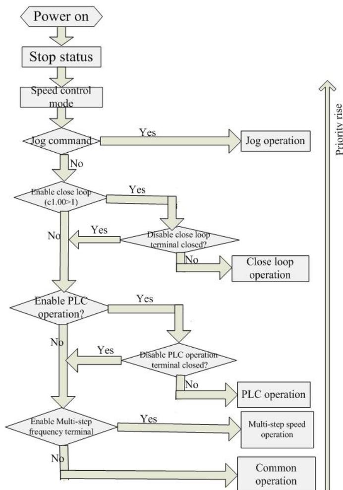
Fig 5-4 Operating mode in speed control mode
