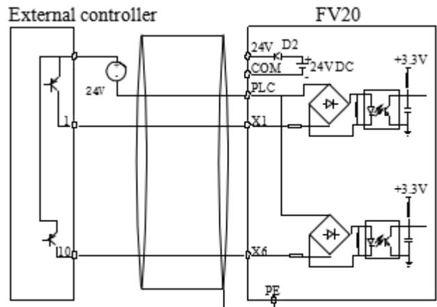
Fig 4-12 Use external power supply for drain connection
