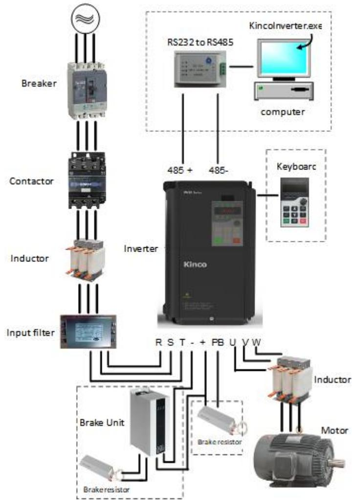
Figure 3-4 Standard peripheral configuration diagram of the inverter
