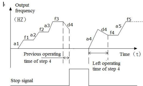
Fig.6-51 Start mode 2 of PLC function
