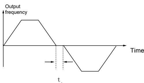
Fig.6-6 Delay time from reverse running to forward running or from forward running to reverse running
