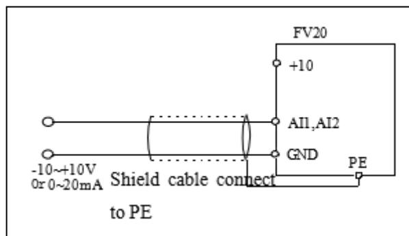
Fig 4-3 AI1 , AI2 terminal wiring
